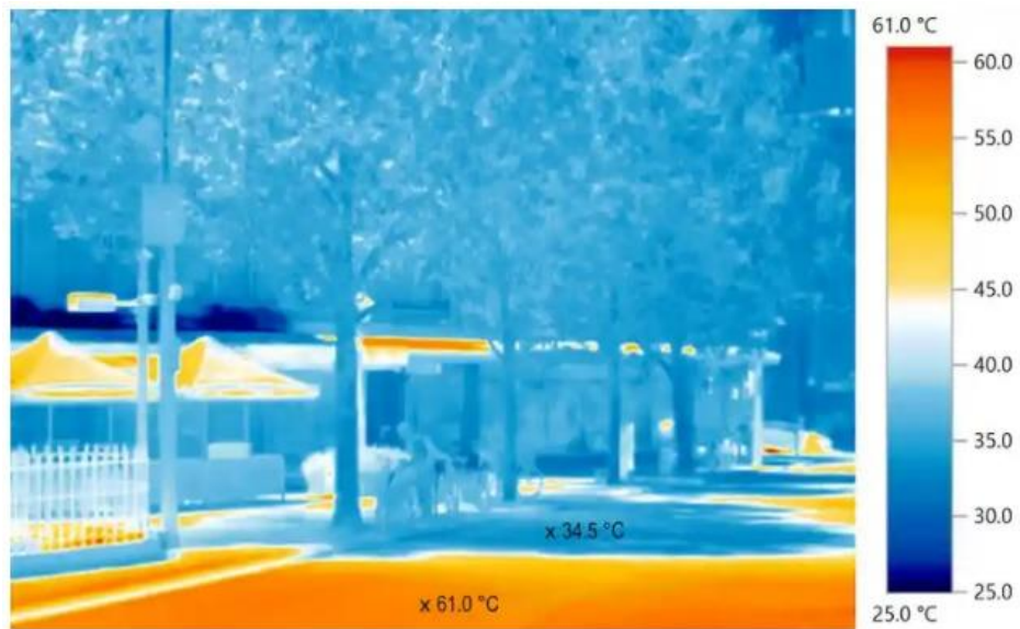
▲ Thermal images taken in a January 2017 heatwave show the impact of urban heat islands in Melbourne. Taken by an Elizabeth Street heat camera opposite Queen Victoria Market. Photograph: City of Melbourne
